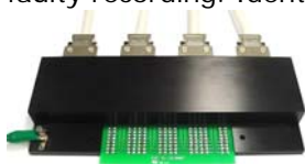
Figure 14. The Test board installed in the MED Multi-well Connector.
