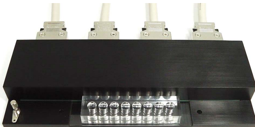
Figure 8. MED Multi-well Connector where Probe is installed.
