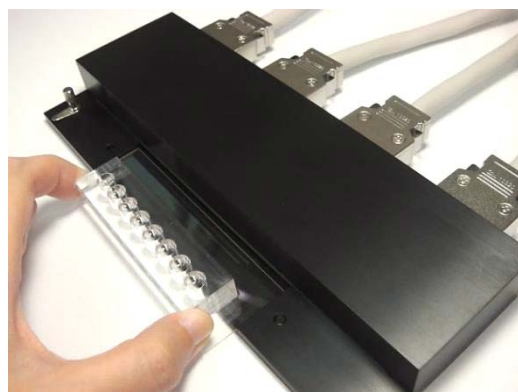
Figure 7. MED Multi-well Probe (MED-5N811) with its terminals on the top (left) and installing the MED Multi-well Probe onto the MED Multi-well Connector (right).
